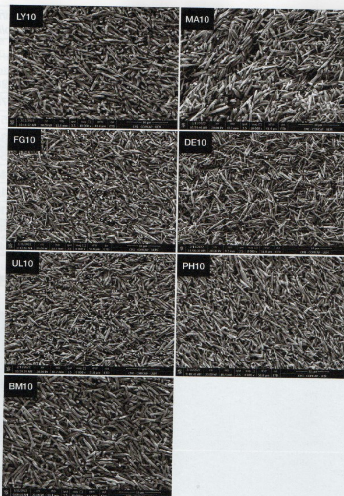
Figure 2. Field-emission scanning electron microscopy images resulting from hydrofluoric acid etching at concentrations ranging from 9% to 10% of various commercial brands. Abbreviations: LY10, Acid Conditioner for Porcelain (Lysanda); MA10, 10% Acido Gel (Maquira); FG10, 10% Condac Porcelana (FGM); DE10, 10% Porcelain Conditioner (Dentsply); UL10, 10% Porcelain Etch (Ultradent Inc); PH10, Potenza Attacco (PHS do Brasil); BM10, 10% Power C-etching (BM4).
